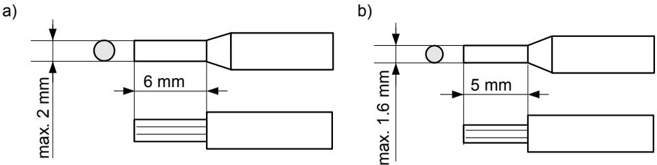
Figure 4.2. Recommended dimensions of cable stripping
