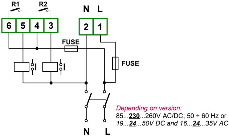
Figure 4.11. Connection of power supply and relays
