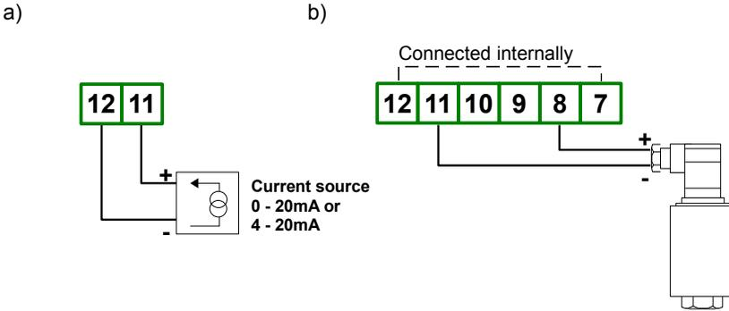
Figure 4.16. Connections of 2-wire sensor:
