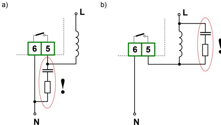
Figure 4.12. Examples of suppression circuit connection:
