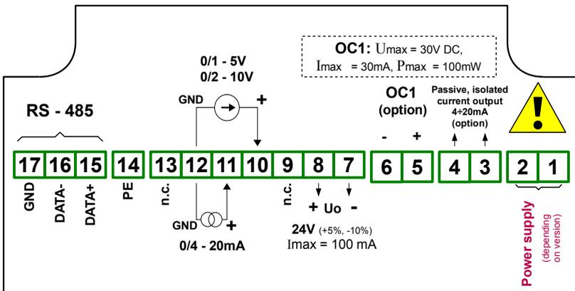
Figure 4.7. Terminals description (OC-type and current output)
