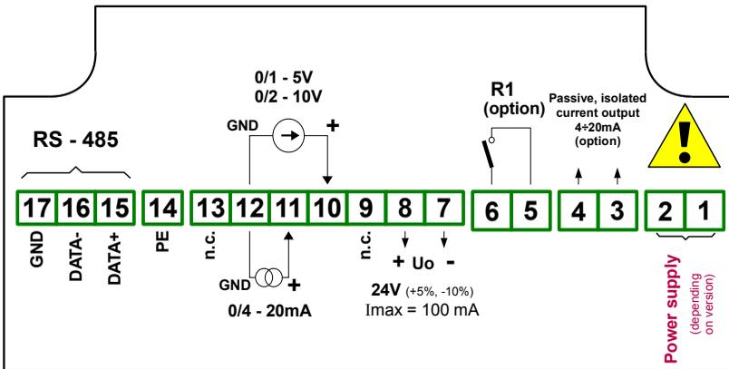
Figure 4.6. Terminals description (relay and current output)
