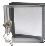
Door and frame are made by injection moulding thus assuring an exact fit, an optimal choice of a material which is very strong and with no risk of corrosion; perfect seal-protective system IP 54 provided by all-round soft rubber sealing the moulding; door does not swing in or out sideways on opening; door-frame and front-frame can be exchanged.
